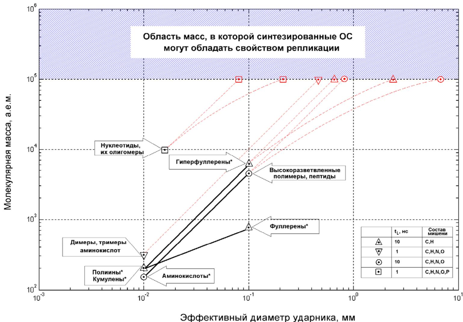
Dependence of mass of OC synthesized in a plasma torch from effective diameter projectile, duration of laser action and the target composition.
