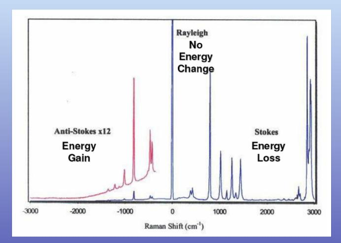
Stokes and anti-stokes Example of Raman cyclohexane spectra
