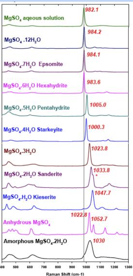
Identification of hydration state of magnesium sulfates by Raman spectrometry. (Wang 2006)
