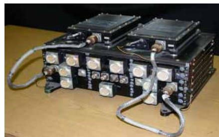
High energy ions spectrometer 10 eV – 50 keV
