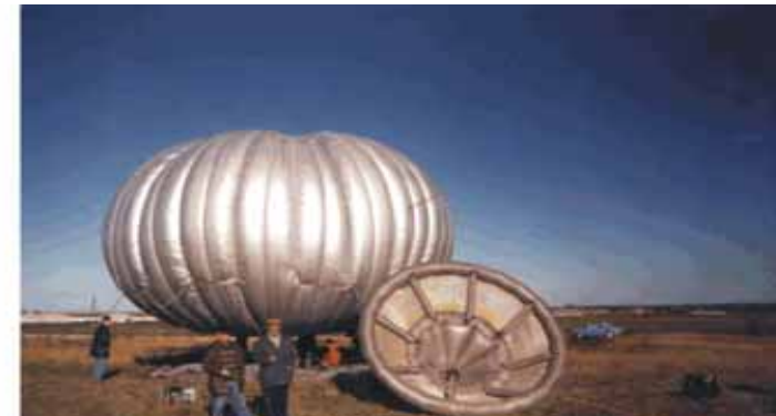
Balloon drop test of the penetrator (penetrator with inflatable braking device)
